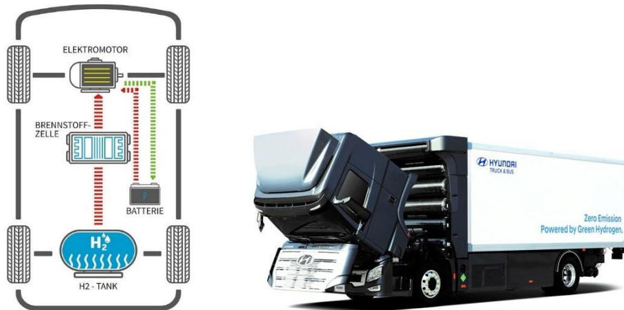
Fig. 2. Schematic diagram of a hydrogen vehicle and a test truck from Hyundai
